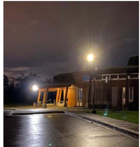
ESD is pleased to announce the installation of 2 solar panel street lights in front of the administration building and cultural centre. The solar panels charge a rechargeable battery, which powers an LED lamp during the night. These lights were designed and developed to provide suitable lighting for low-lit areas around the buildings and to help in reducing energy consumption, which helps offset and conserve energy use that is required to power the infrastructure.
