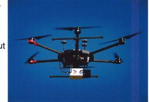
The drone being flown in July uses <u>LiDAR</u> technology to map the land by collecting surface information about the shape of the land and trees, as well as plotting the roofs of buildings and other structures. According to UBC, the LiDAR data will be collected at night when there are few people or moving vehicles out.
