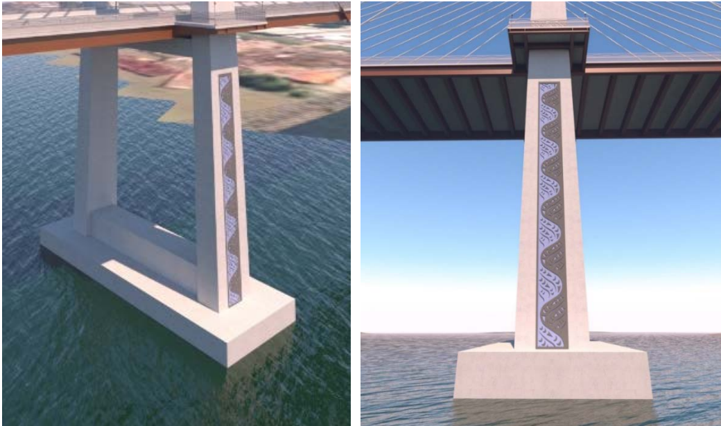
Figures – Example of linear lower tower leg embossing starting directly above pile cap
