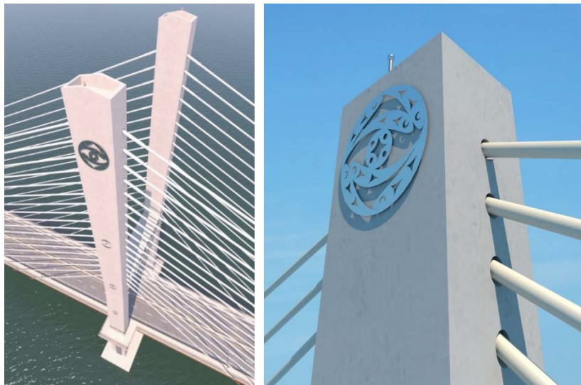
Figure – Example of primary medallions attached to upper legs of tower
