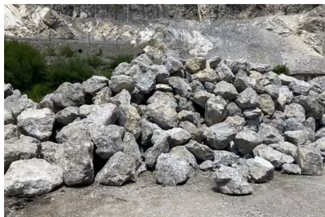
Example of new riprap rock material to be installed as erosion protection. This type of riprap will replace the existing concrete at the Musqueam foreshore. Photo provided by Core Project Management.
