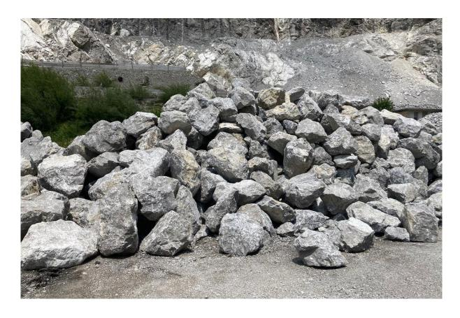
Rip rap material to be installed as erosion protection
