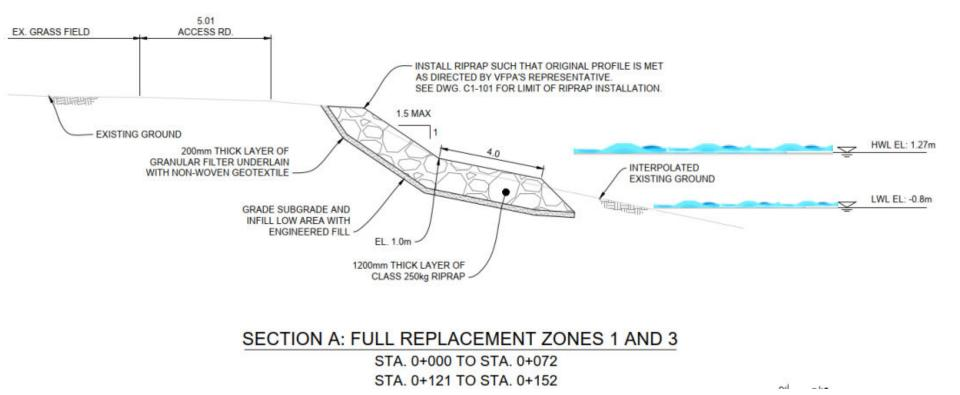
Majority of the work will include **full replacement** of existing concrete debris with engineered rip rap erosion protection.
