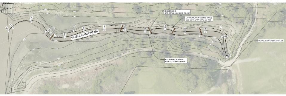
Enhancements will include a series of log structures as an alternative to the rock weirs – known as 'Digger Logs'.
