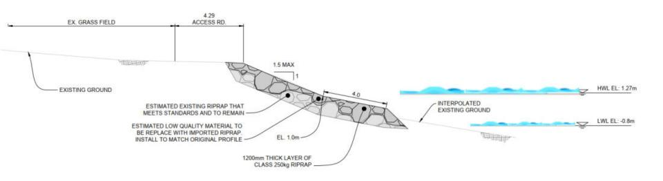
SECTION B: PARTIAL REPLACEMENT ZONE 2 STA. 0+072 TO STA. 121
