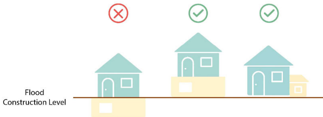
Figure 4. Examples of Buildings that Do and Do Not Comply with Flood Construction Level Requirements
